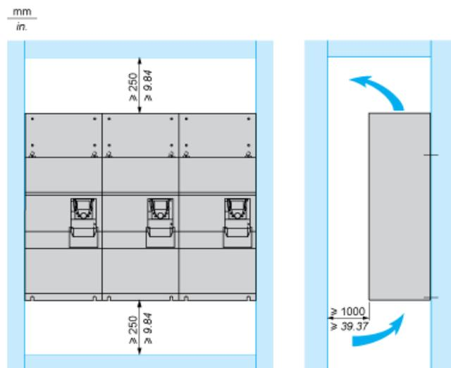
Specific Recommendations for Mounting the Drive in an Enclosure
